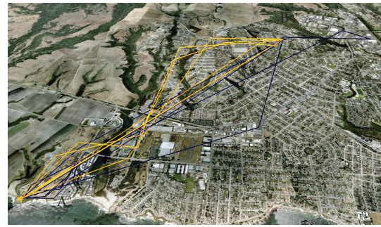
FIGURE 18: GPS data from the test deployment. The yellow track was logged by the GPS on a CSN carried by a researcher. The black track is the GPS data from the CSN carried by a domestic dog. An SRN was located at Long Marine Lab, Santa Cruz, CA, USA (A). The dog lived at B and his owner worked at A. Data was successfully transferred to the SRN via hops 1 and 2.
